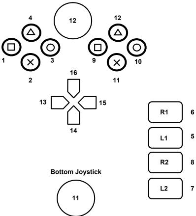
The Shoulder buttons, L1, L2, R1, R2, are implemented on the back spine of the handset, and are labelled up as per the format of the SONY PS3 handset.
